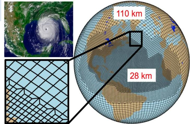
Variable-resolution grid of the model CAM5-SE that bridges the grid spacings 110-28 km in a single AMIP simulation. \
